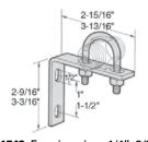
Part# 11543: For pipe sizes 1/4", 3/8" and 1/2" Part# 15542: For pipe sizes 3/4" and 1" U-Bolt# 11040
