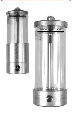
Designed to be placed between the valve and cylinder in a pneumatic circuit, Monnier's Air/Oil reservoirs provide the predictable, even cylinder actuation of a hydraulic system in a low cost pneumatic circuit.
